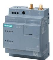
LOGO! CMR2040 communication module for connection LOGO! 8 to LTE network; 1 RJ45 port for Ind. Ethernet connection to LOGO! 8; 2xDI; 2xDO; write/read access to LOGO! variables; SMS dispatch/ receiving of text messages; email dispatch; position detection GPS; time synchronization/ forwarding with real time clock; Configuration/diagnostics via web interface; Remote access via OpenVPN/HTTPs, DynDNS, observe national approval! Manual available as a download.
